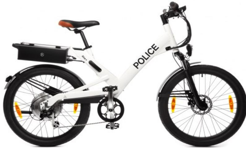
An electric bicycle, also known as an e-bike or booster bike, is a bicycle with an integrated electric motor which can be used for propulsion. There are a great variety of e-bikes available worldwide, from e-bikes that only have a small motor to assist the rider's pedal-power (i.e., pedelecs)
